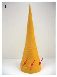
Locate slots at the base of the cone. This will determine the cross-section of your O-Ring.
