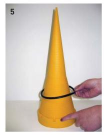
In this example, we have determined that the O-Ring is a member of the -400 series. Slide the O-Ring down the cone until it comes to rest on a step. Do not apply any unnecessary force!
