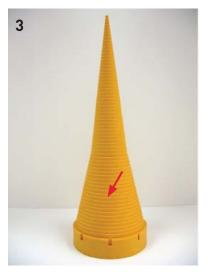
The raised numbers above the chosen cross-section slot will determine the "series" your O-Ring belongs to.
