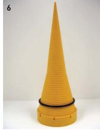
Read the O-Ring size from the step it is resting on. In this example, it is resting on the step between 428 and 430. Therefore, the size is 429.
